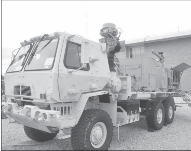
Figure A-15. Tactical communications node
